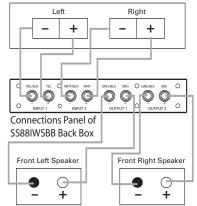
using a dedicated subwoofer amplifier or your main receiver/ amplifier to power the SS88IWS, select one of the two connection methods that follow.
